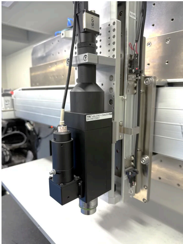
USB 3 uEye CP industrial cameras from IDS are the sharp eyes of the uLED laser soldering machine from MSP.
