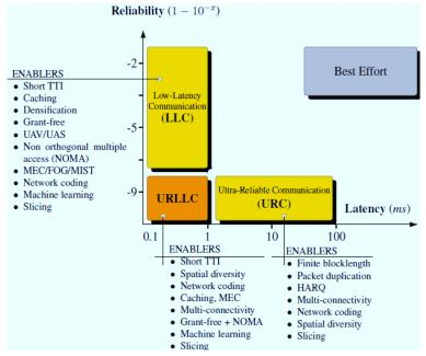
Figure 4-14 Enabler for low latency and low reliability
