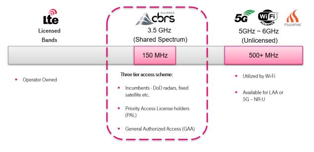
Figure 3-3 CBRS 3550-3700 MHz Spectrum Framework
