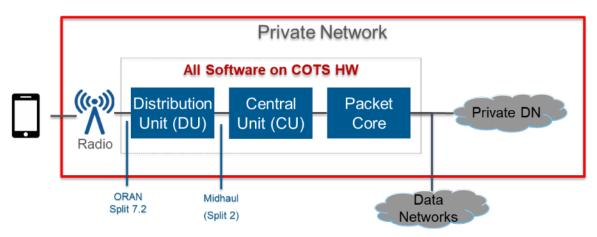
Figure 4-11 ORAN (or vRAN) Deployment for NPN
