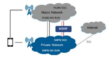
Figure 4-7 Access to SNPN services via PLMN vs direct access to SNPN
