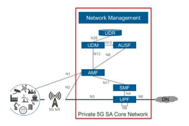
Figure 4-8 Stand-Alone 5G NPN – Reference Point Architecture
