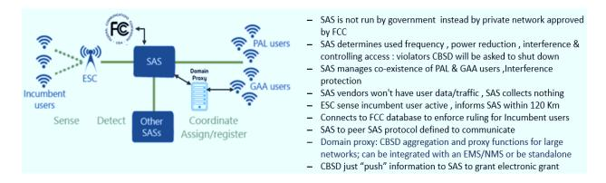
A high-level view of CBRS spectrum sharing system is given in Figure 5-1.
