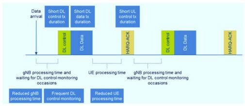
Figure 4-16 Enabler for low latency
