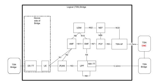
Figure 4-18 System architecture view with 5GS appearing as TSN bridge
