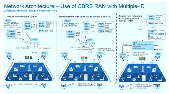
Figure 5-3 CBSD end to end deployment models
