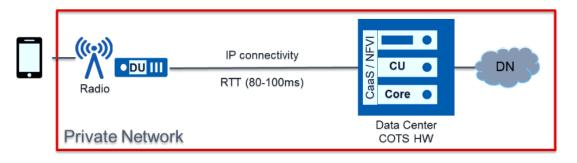
Figure 4-12 Latency constraints for NPN in RAN split topology
