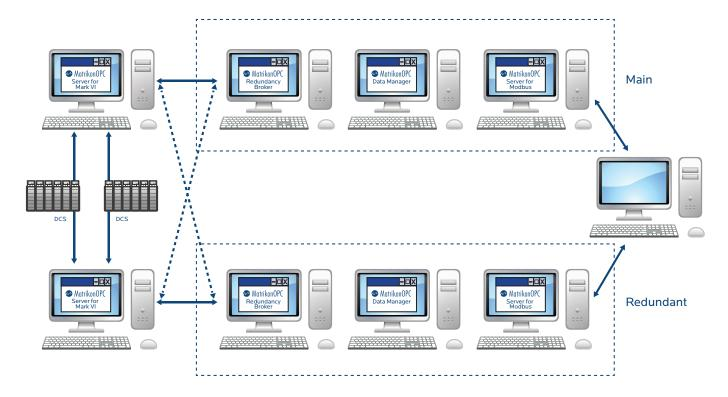
As the name implies, this model applies redundant software and communication channels at the three major levels of the architecture; the OPC client application, the OPC server and the end device or data source.
