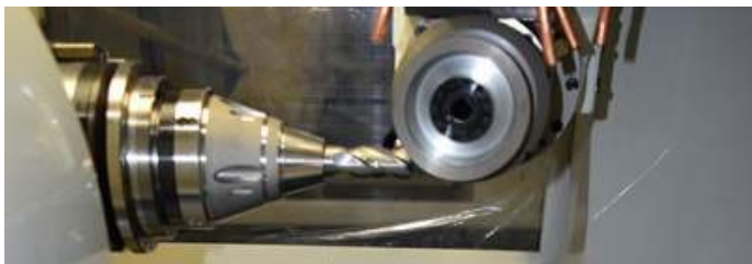
The linear motor is very compact under the way cover and a voids ball screw stick-slip and wear issues while providing 10 percent faster cycle times.
