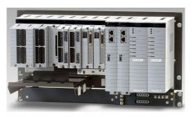
The newly developed FCS (FFCS-V) builds upon the high reliability of the CENTUM "Pair & Spare" methodology providing, an availability of 99.99999 percent when configured with dual-redundancy. Each control processor has redundant CPU's that execute the same control computations simultaneously and then their outputs are compared. Assuming the outputs are equal, the main processor outputs to the final control
