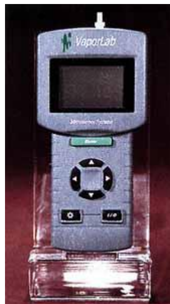
Photo 2. A commercially available handheld SAW chemical vapor analyzer incorporates an array of four SAW sensors, each coated with a different polymer.
