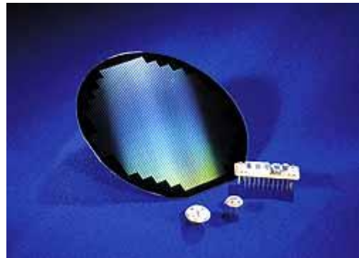
Photo 1. Acoustic wave sensors are commercially available in several form factors. Most sensors begin as processed wafers that are then tested, diced, and mounted into packages.
