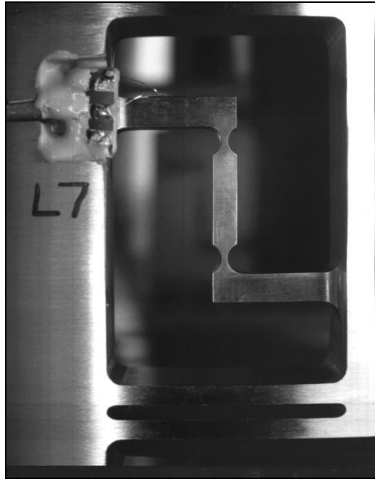
Figure 7.- Bending beam arrangement
