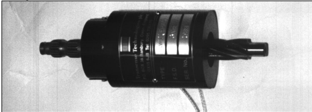
Figure 5.- Prototype SAW Torque Transducer
