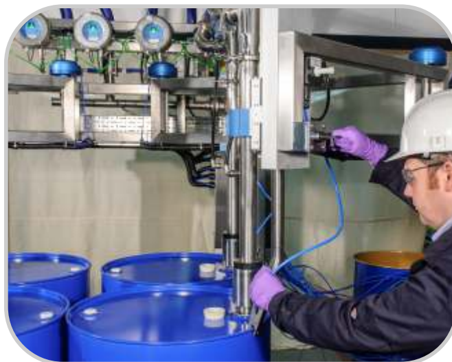
Fig. 2: pulsing green ground status indicators provide operators with a visual reference point to ensure the equipment they are operating is grounded prior to, and during, the operation.
