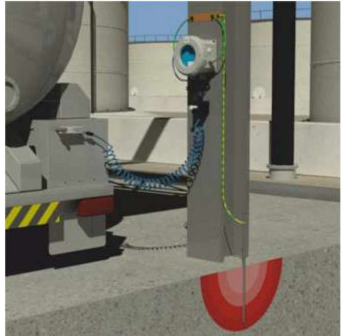
Figure 2: Verified ground electrodes are critical to ensuring static electricity is removed from the HAZLOC area. Concentric shells of resistance present around the ground electrode can impede the flow of electrical currents, regardless of whether they from electrostatic, lightning or electrical fault sources.
