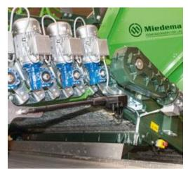
Two LINAK electric actuators adjust the roller technology exactly to set measurements between 5 and 65 millimetres. The entire mechanism is protected by precise positioning and not strained beyond the recommended limit. Due to the <u>communication</u> between the two LINAK electric actuators, a parallel displacement is guaranteed and is recognized as a big plus for an even grading over the 2.40 meters width of the cleaning and sizing rollers.
