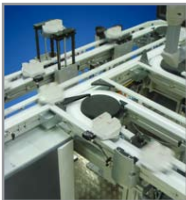
Individual work stations for manual or automatic operations, testing etc can easily be added to a line.
