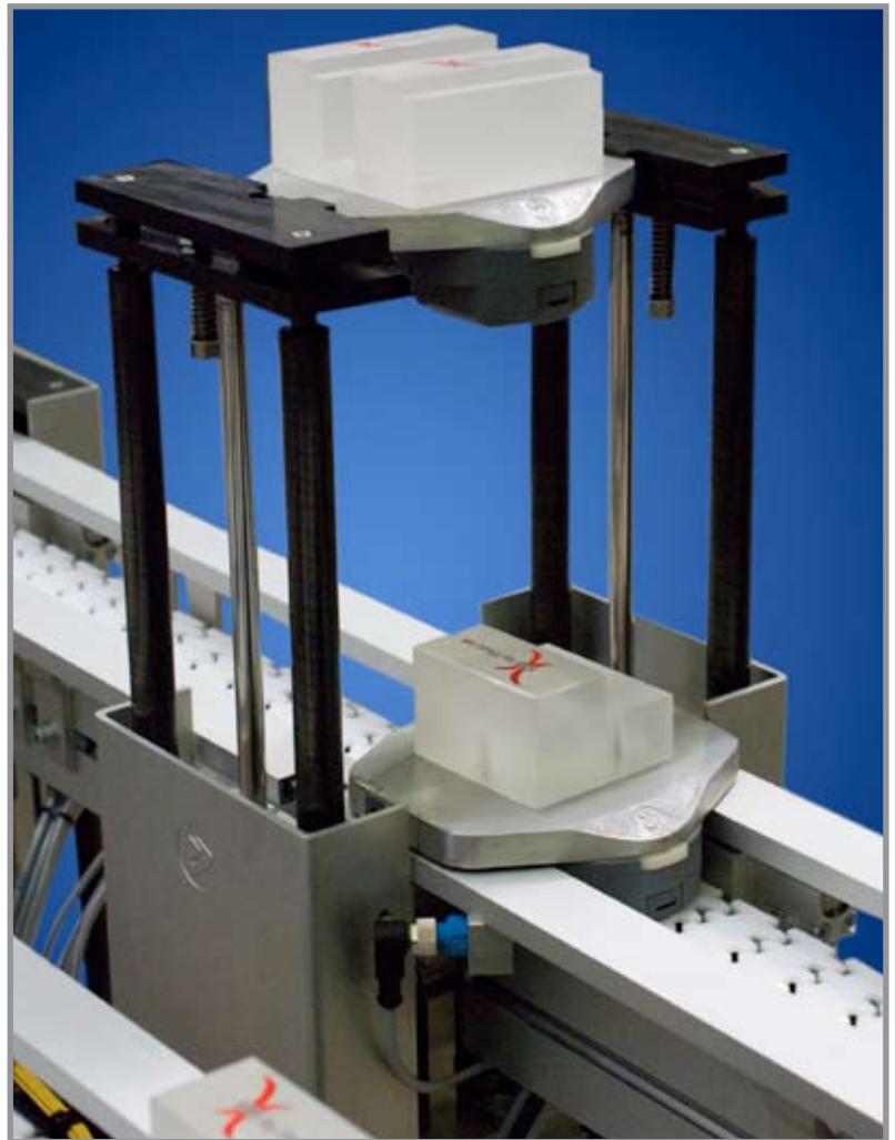
Tunnel locating modules can in pair serve one robot, or machine, enabling continuous operation – highest possible utilization of the equipment.
