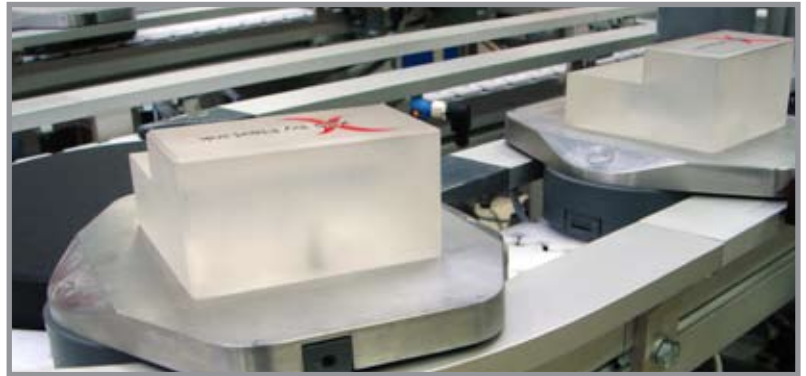
The pallet is prepared for RFID communication with the line control and MES system. Tunnel locating modules can in pair serve one robot, or machine, enabling continuous operation – highest possible utilization of the equipment.
