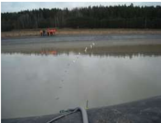
Fig 3: The robot in operation in the PV pond. In the foreground, on the pond's edge, are seen the electric cable and the hose fitted with buoys to assist the remote control of the robot.
