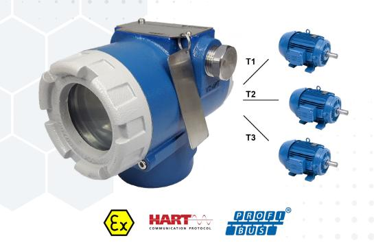
VTT10-F is a temperature transmitter for field mounting with a multifunctional LCD display. It accepts TC, RTD, Ohm and mV sensors, generating a 4 – 20 mA current signal (HART® 7 model) or a digital signal (Profibus-PA model), according to the measurement type and user configuration. The Profibus-PA line has 2 or 3 channel models (VTT10-FP3), and the 3-channel is ideal for temperature measurements in motors.
