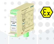
VTT10-P is a temperature transmitter for DIN rail mounting, that accepts TC, RTD, Ohm and mV sensors, generating 4-20 mA current signal (HART® 7 model) or a digital signal (Profibus-PA model), according to the measurement type and user configuration. The HART®/4-20 mA model has two open-collector outputs for alarms or on/off signals.
