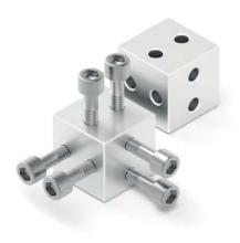
This is a QB - a simple, versatile aluminum cube with a 10mm or 0.5" side. Each face of the QB has a pair of mounting holes with a distance of 5mm or 0.25" between them. All holes are through holes, oriented in such a way that they do not intersect within the QB.
