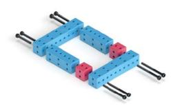
Use plain QBs to turn any beam (and beams always come in odd sizes) into an even-sized "beam". For example, take two BMC-3s, two BMC-5s, and two plain QBs to construct a 5x6 rectangle.
