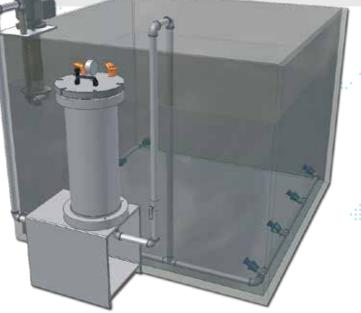
CTV is commonly installed in surface treatment baths, circulating through filter and further to nozzle ramps.
