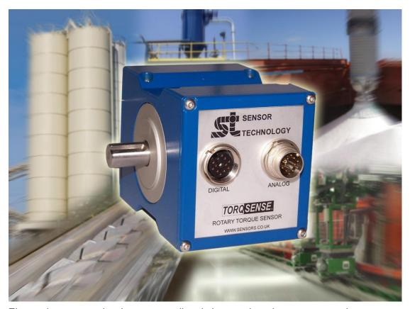
Electronics convert the data stream directly into engineering outputs, such as torque, speed, power and angle. Serial and USB interfaces make TorqSense directly compatible with PCs and other user-friendly features include built-in peak torque sampling, storage and torque averaging, and a self-diagnostics test package. The electronics can be provided, integral with the main unit or in a separate housing, to suit individual applications.
