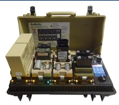
Fast Charging: 8 BB-2590/U Batteries Charged From 0% to Full in Less Than 3 Hours 16 Conformal BB-2525/U Batteries Charged in Less Than 3.5 Hours
