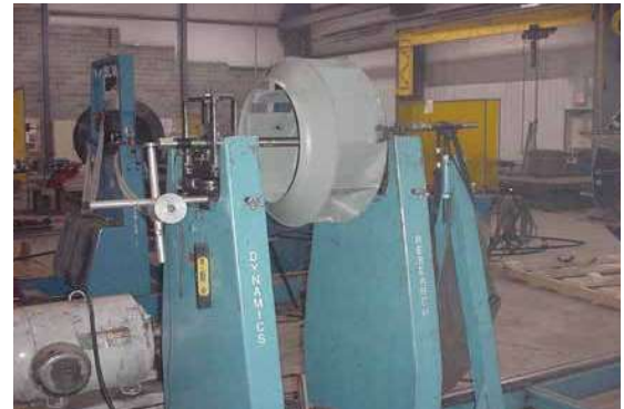
25" backward inclined wheel is being balanced using a mandrel, on our small dynamic balancer with a capacity up to 5,000 lb weight and 100" diameter.
