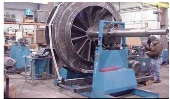
103" radial blade wheel and shaft assembly with chromium carbide liners, A514 steel and chromium construction. It is shown being balanced on our large dynamic balancer with a capacity up to 20,000 lb weight and 140" diameter.
