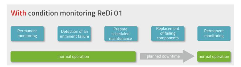
ReDi 01 is an intuitive user friendly remote diagnostics tool enabling predictive maintenance running under Microsoft® Windows® on Skylake based MSC systems. It minimizes the time the equipment is being maintained, the production hours lost to maintenance, and the cost of spare parts.
