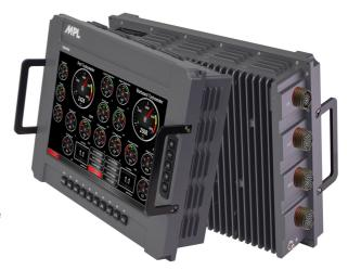
The system is designed with a military grade, high strength, and light weight housing (SWaP-C). The enclosure meets IP54 all around. Its modular architecture allows the system to be easily configurable with many options (GPS, 1553, WLAN, LTE...). Additional function keys for faster operation of the system can be implemented. An expansion with GPU for compute-intensive applications such as image processing, can easily be integrated.
