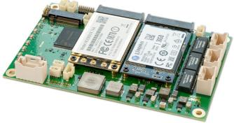
The internal two miniPCIe slots and the M.2 slot allow various extensions (WLAN, GPRS, LTE, mSATA SSD, ...). The  $\mu$ GUARD is available as OpenFrame on a cooling plate to be mounted in existing housings or cabinets. Fiber can be provided over an additional modul (TX2FX). Alternatively MPL offers a firewall solution with RJ45, M12, or MIL-38999 connectors. The standard operation temperature range is -20°C to +60°C and is optionally available in extended temperature of -40° up to +85°C.
