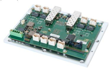
The input power requirement of the device is 8 - 36VDC and comes with reverse polarity protection (optional with redundant input) and less then 15W power consumption at full operation. The product can be operated at -20°C up to +60°C.
