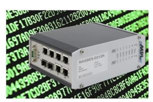
dundant power input, galvanic isolation or different power input ranges) and uses under any condition less than 8W (5-port switch less then 4W). Optional available is also coating and bonding.
