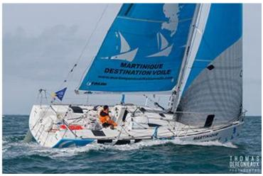
windy conditions. Its wide hull and its double rudders, combined with an extremely strict weight specifications allow it to reach very high average speeds especially downwind, and the same under autopilot.
