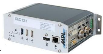
For the temperature tests, the Class Tx has been chosen, which means -40°C to +70°C and +85°C for the duration of 10 minutes. For shock and vibration, Class 2 (Bogie mounted) has been selected which the second most severe vibration test standard in the railways industry. The tested products are ready to be delivered.
