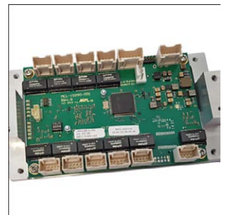
Customized 10-port Gigabit switch with cooling block
