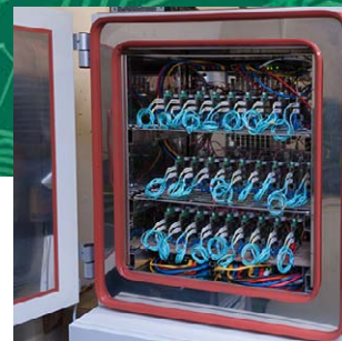
MPL climate chamber test environment
