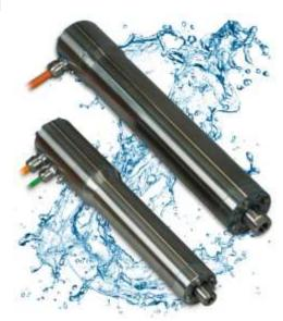
The hygienic IMA-S series servo actuator offers forces up to 11.1 kN (2500 lbf), stroke lengths up to 450 mm (18 inches) and options for planetary roller screws or ball screws. A proprietary lubrication feature helps extend service life.
