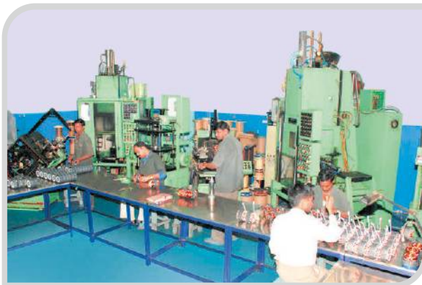
Semi Automatic Winding Line for Stator Production
