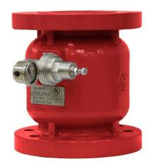
Without external conduit, Z-Tide (axial) piston type valves are easier to transport, install and maintain. The compact cylinder design and straight flow path with large flow capacity would reduce malfunctions and decrease turbulence. Pressure drop is tested at ratio 6:1 without cavitation.
