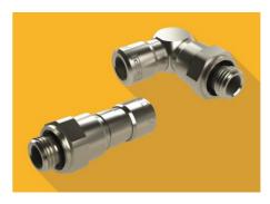
This new push-in connector from series 14 of the BASICLINE is the first fully rotating connector in Eisele's product spectrum. The rotary movement is enabled by a hybrid stainless steel ball bearing with ceramic balls, which is approved for rotational speeds of up to 800 rpm. Stainless steel versions that are suitable for other operating media will follow.
