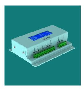
Supports all Datum Inline and Shaft Power Measurement Solutions Displays; Torque, Speed RPM, Power and Status Operating Range: -10 to +70 °C ( +14 to +158 °F) Environmental Protection: IP54 Analogue Outputs: 4-20mA, +/-10Vdc, +/-5Vdc, 0-10Vdc or 0-5Vdc Digital Outputs: RS485, RS232. Ethernet, USB Type Mini B, USB Type A Also accepts an input from an external shaft speed tacho Power Supply: 15-24Vdc (included)
