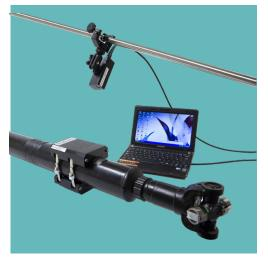
Shaft Sizes: 90 - 1,100 mm (3.5433 " - 43.3071 ") Accuracy: +/- 0.1% Battery Life: 30 days (charger included) Operating Temperature: 0 to + 70 °C ( +32 to + 158 °F) Data Sampling Rate: 10 sps as standard (for 100 sps contact sales) Cable Length: 10m as standard Data Output: RS485 to DUI Single or Dual Channel Strain PC Software
