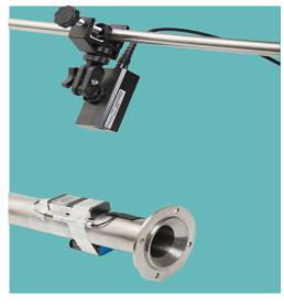
Shaft Sizes: 30 - 500 mm (1.1811 " - 19.685 ") Accuracy: +/- 0.1% Battery Life: 30 hours (4 days) Operating Temperature: 0 to + 70 °C ( +32 to + 158 °F) Data Sampling Rate: 10 sps as standard (for 100 sps contact sales) Cable Length: 10m as standard Data Output: RS485 to DUI Single or Dual Channel Strain PC Software
