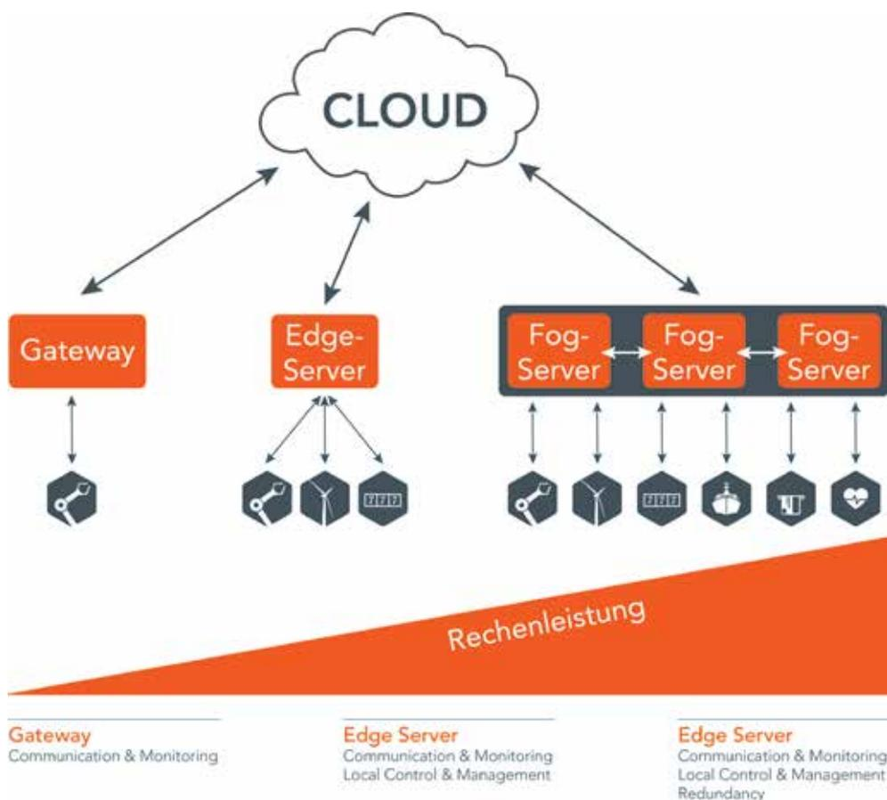
In addition to the bridge functions of gateways, edge and fog servers also provide complete control and management of applications locally.
