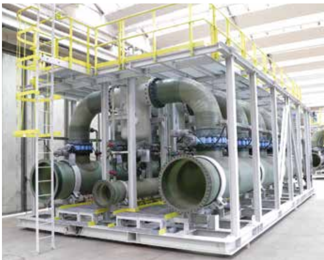
Automatic Filtration System
