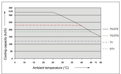
Remark: The limit curves for the heat exchangers exchanger apply to a dew point of 65  $^\circ$ C.
