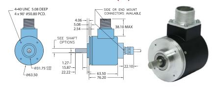
All dimensions are in mm with a tolerance of ±0.127mm or ±0.254 unless otherwise specified
