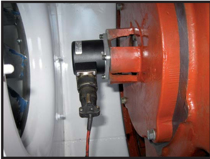
An BEPc Size 25 Encoder in a common application.
