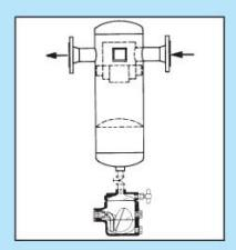
**Function** - BEP high efficiency moisture Separators are specifically designed for the extraction of liguid particles from air/gas flow.
