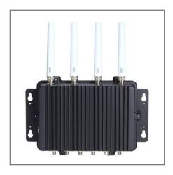
Axiomtek's eBOX800-511-FL with high reliability and stability can be installed on Rotary Mining Drill as a collision avoidance system which is 24/7 in operation. The embedded system features fanless operation, wide operating temperatures and rugged housing to enhance the system stability for use in mining. Moreover, the eBOX800-511-FL also can be installed in tank truck or heavy-duty industry as the surveillance application.
