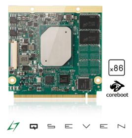
Qseven<sup>®</sup> is an off-the-shelf, multi-vendor, computer-on-module that integrates all the core components of a common x86 PC and is mounted onto an application specific carrier board. A single ruggedized 230-pin MXM connector provides the carrier board interface to carry all the I/O signals to and from the Qseven module.
