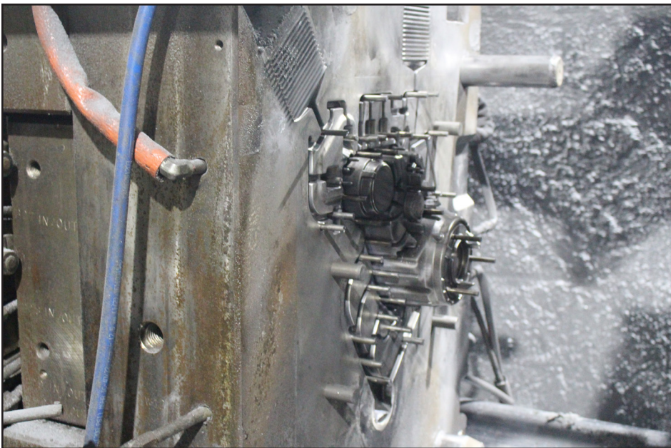
Figure 2-9 Ejector half of the die with the ejector pins extended.
