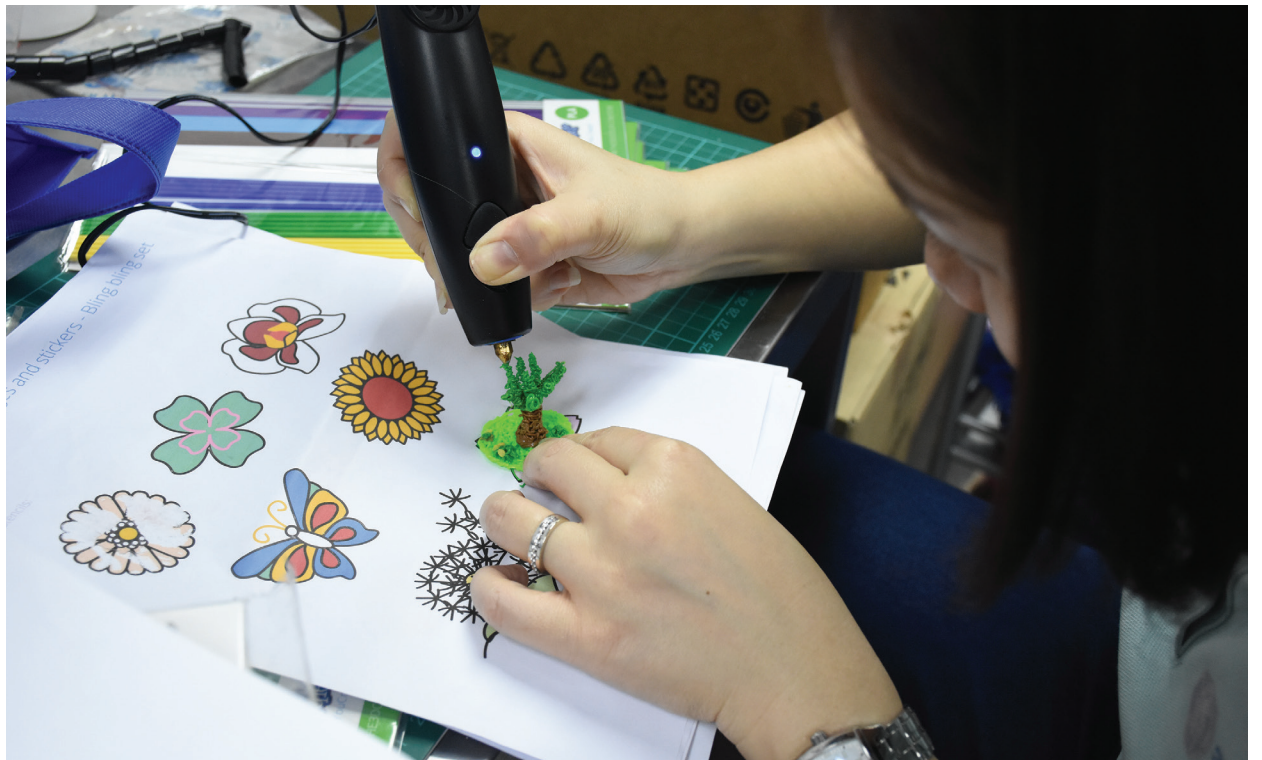
A 3D printed object is created by laying down successive layers of material until the entire object is created. The materials are deposited layer by layer, as liquids, pastes, or powder, and are fused using heat or light.
