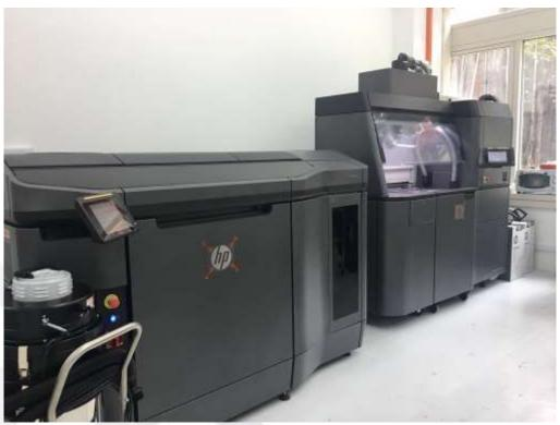
The new HP Jet Fusion 3D Printing solution within 3D Matters' Additive Manufacturing Centre located at Singapore Science Park II. The system comprises of a printing unit (left of picture) and a processing station (right) that support successive and multiple print runs to maximize productivity.
